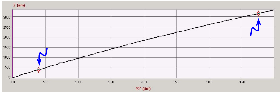
Figure 9-4 Vertical cross-section of the 10% sloped surface.
